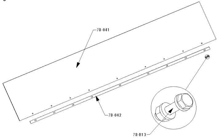
Screener Model SLG 78VF SLG 78 Screen Deck Assembly Page 006-D
