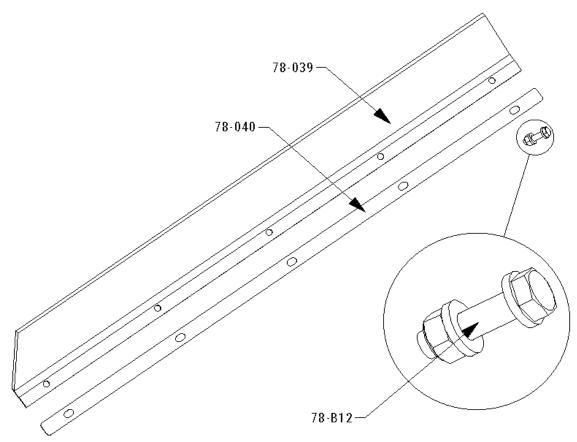
Screener Model SLG 78VF SLG 78 Screen Deck Assembly Page 006-C
