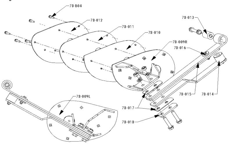
Screener Model SLG 78VF SLG 78 Screen Deck Mount Assembly Page 002-A
