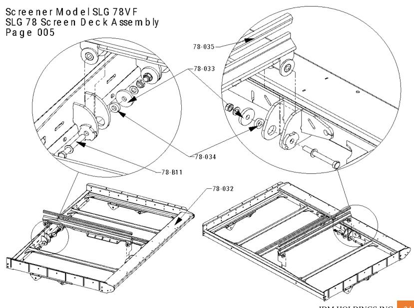
Screener Model SLG 78VF SLG 78 Screen Deck Assembly Page 005-A
