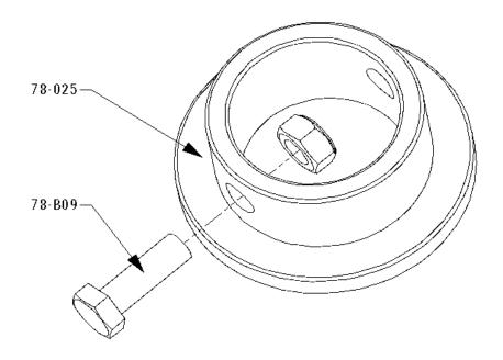
Screener Model SLG 78VF SLG 78 Coil Spring Assembly Page 003-B
