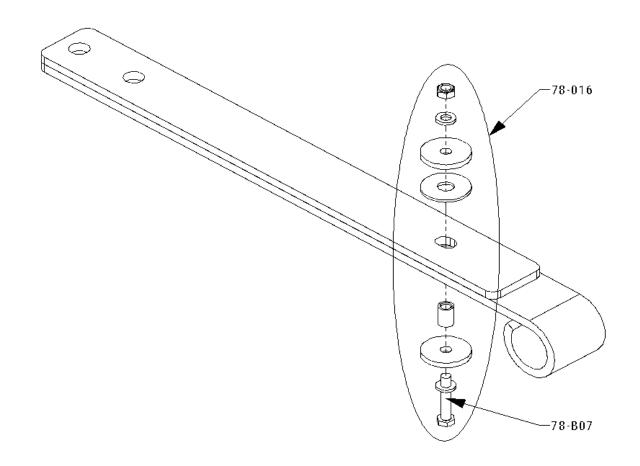
Screener Model SLG 78VF SLG 78 Screen Deck Mount Assembly Page 002-D
