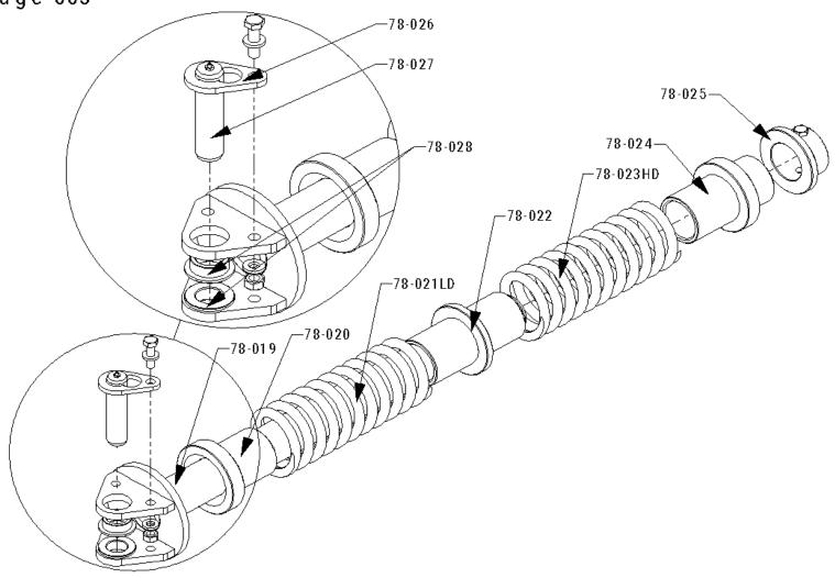
Screener Model SLG 78VF SLG 78 Coil Spring Assembly Page 003-A
