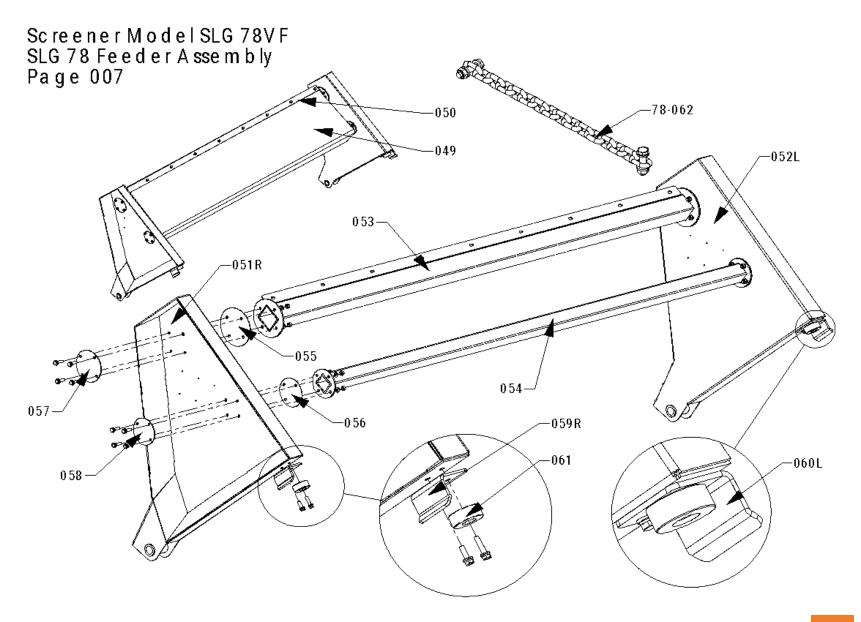
Screener Model SLG 78VF SLG 78 Feeder Assembly Page 007-A
